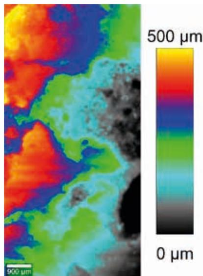
**Figure 3: Topography of the sample.** Recorded using the TrueSurface® extension of the alpha300 microscope series.
